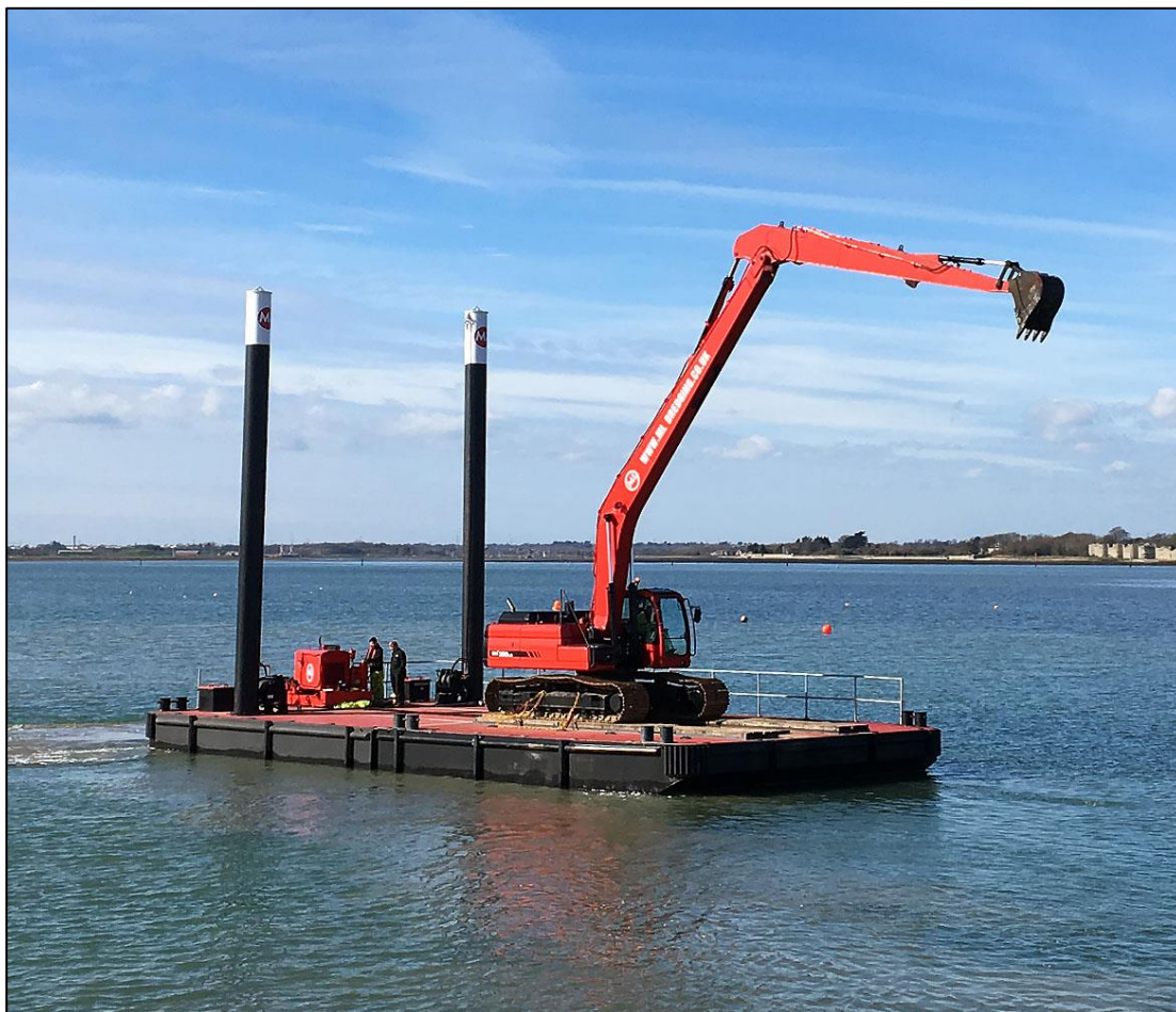
Plate 11.16 Example of Spud-can Barge with long-reach excavator to be used in the construction of the works.
